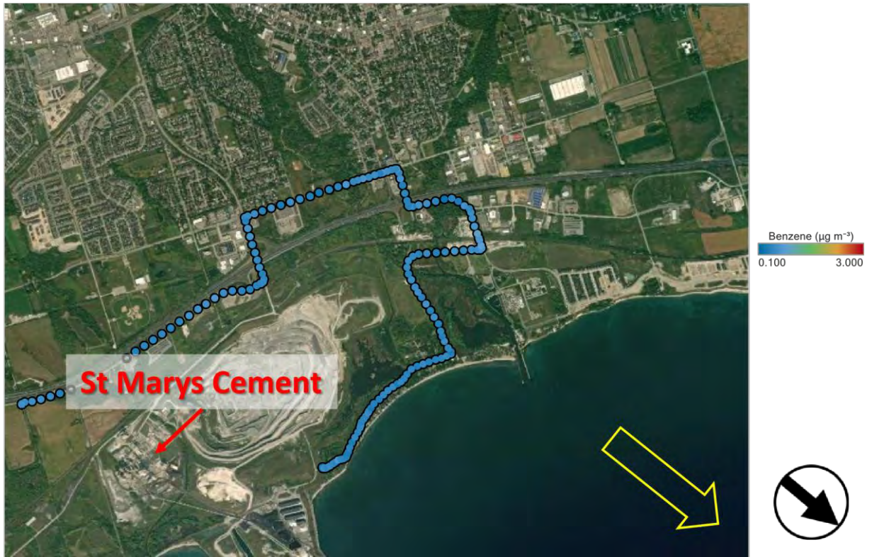
Figure 2: Mobile monitoring of benzene in the vicinity of the St. Marys Cement plant, Municipality of Clarington, Ontario, July 22, 2021 10:20-10:40. The red arrow indicates the general location of the facility. The yellow arrow indicates the direction the wind was blowing during the measurement period.
