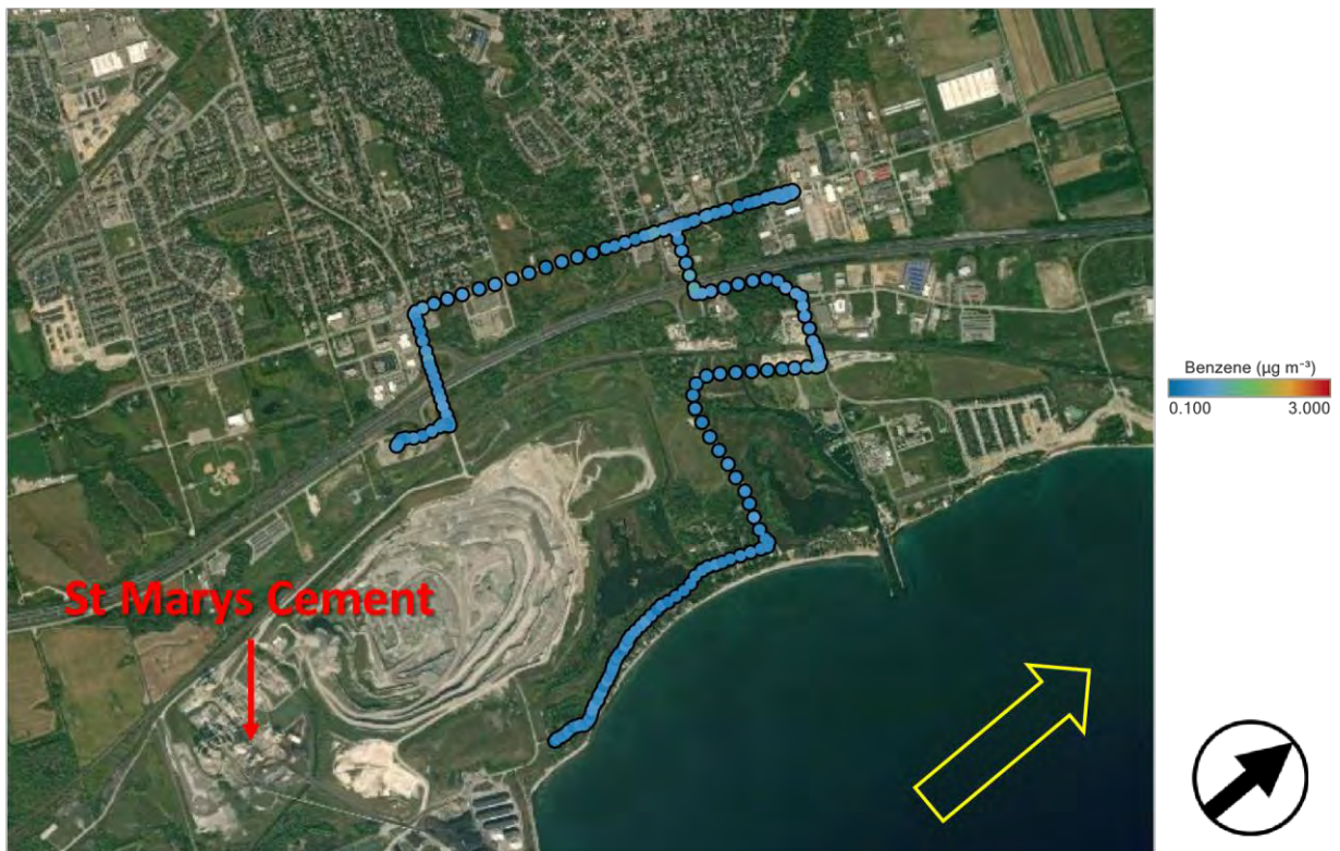
Figure 1: Mobile monitoring of benzene in the vicinity of the St. Marys Cement plant, Municipality of Clarington, Ontario, July 21, 2021 09:47-10:06. The red arrow indicates the general location of the plant. The yellow arrow indicates the direction the wind was blowing during the measurement period.
