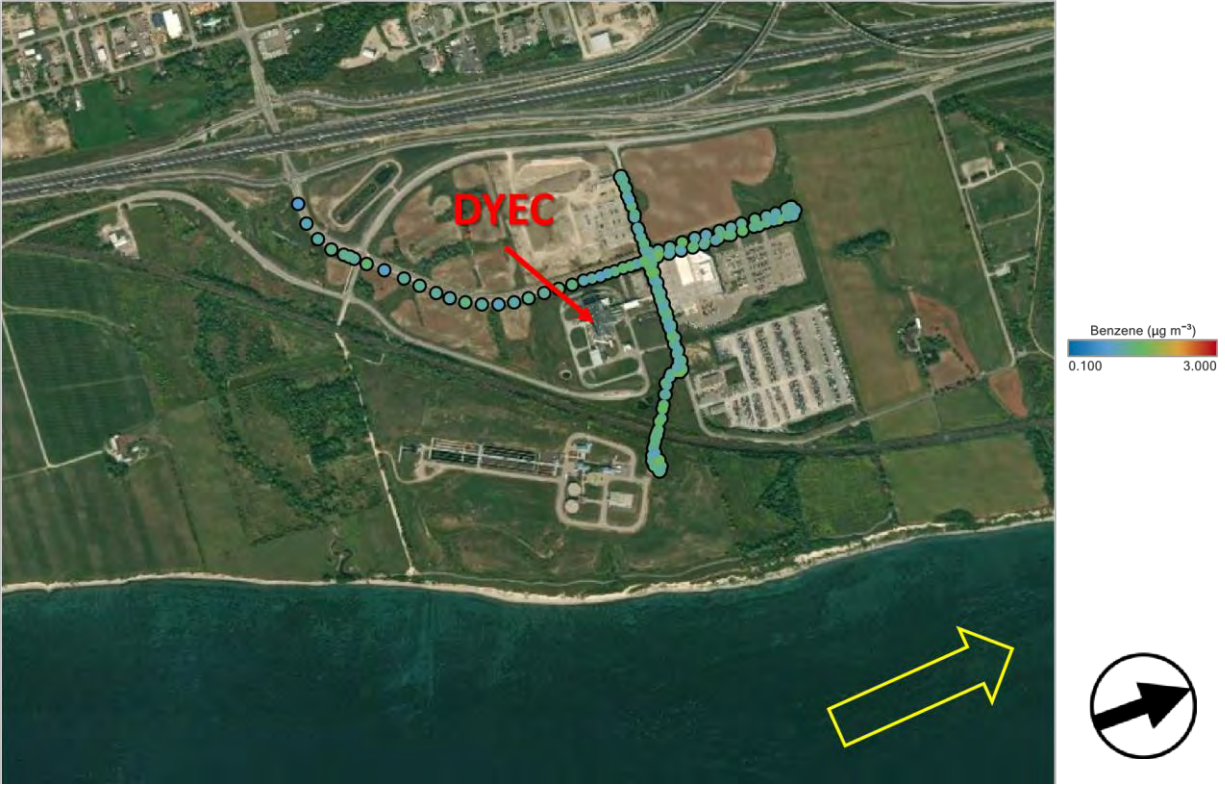
Figure 3: Mobile monitoring of benzene in the vicinity of DYEC, Municipality of Clarington, Ontario, July 26, 2021 11:01-11:12. The red arrow indicates the general location of the facility. The yellow arrow indicates the direction the wind was blowing during the measurement period.
