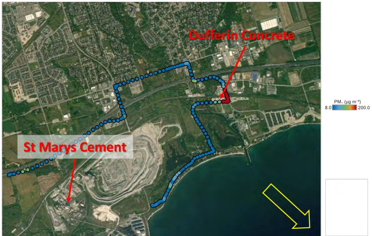
Figure 6: Mobile monitoring of PM 10 in the vicinity of the St. Marys Cement plant, Municipality of Clarington, Ontario, July 22, 2021 10:20-10:40. The red arrow indicates the general location of the facility. The yellow arrow indicates the direction the wind was blowing during the measurement period.
