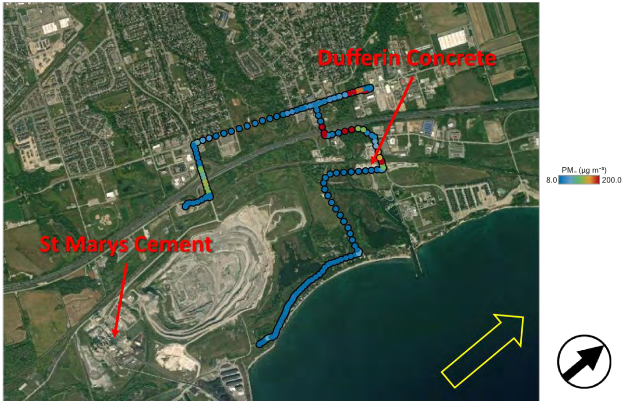
Figure 5: Mobile monitoring of PM 10 in the vicinity of the St. Marys Cement plant, Municipality of Clarington, Ontario, July 21, 2021 09:47-10:06. The red arrow indicates the general location of the facility. The yellow arrow indicates the direction the wind was blowing during the measurement period.
